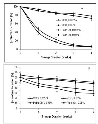
Figure 2. Chemical stability of  $\beta$ -carotene loaded microemulsions during ambient temperature storage. Without (A) and with (B) heating treatment (oven, 105°C for 5 h) prior to storage.
